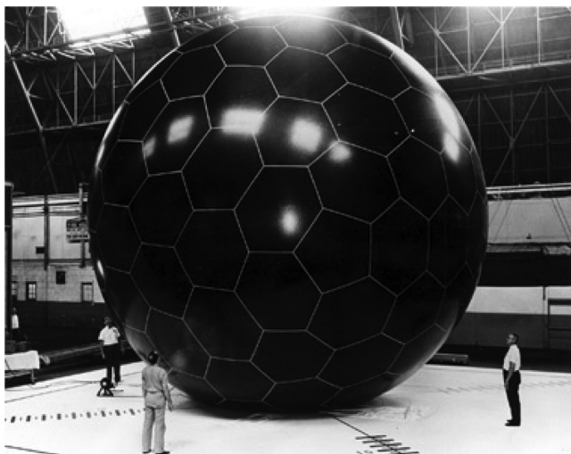
Fig. 19 The OV1-8 satellite with photolysable inflatable bladder embedded in a wire frame mesh (image credit: USAF).
